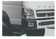
07 Headlamp levelling provide optimum headlamp and light projection distance. Comes with day time running lamp.
