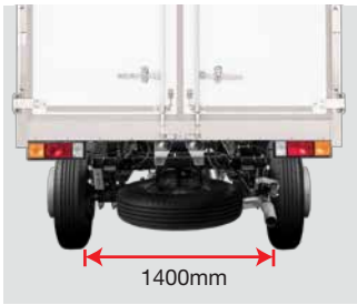
07 1400mm wide rear tread allows installation of higher and wider cargo bodies.
