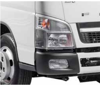
06 Headlamp levelling provide optimum headlamp and light projection distance. Comes with day time running lamp.
